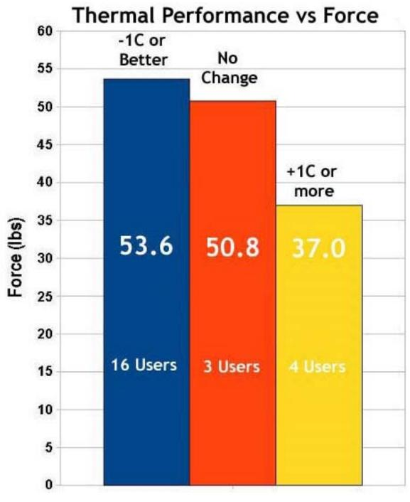
The test involved inserting pressure sensitive film to record mounting force between the heatsink and CPU after installing the heatsink on the CPU. The film records pressures on the IHS from 28 to 98 pounds, which is translated into data, two and three dimensional images by Sensor Products for analysis.
