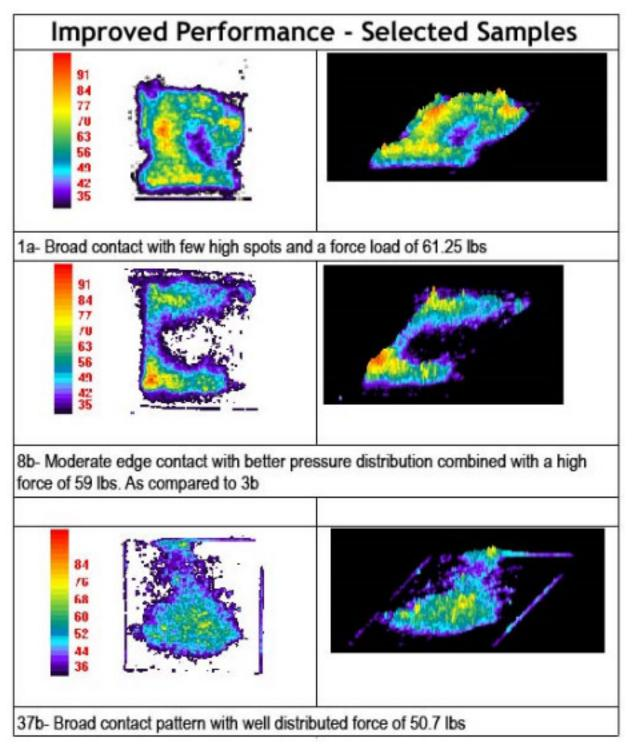
Three users experienced no change even though they had adequate force with an average of 50.8 lbs. Closer examination of the images show uneven contact, with most of the force applied on the edges:
