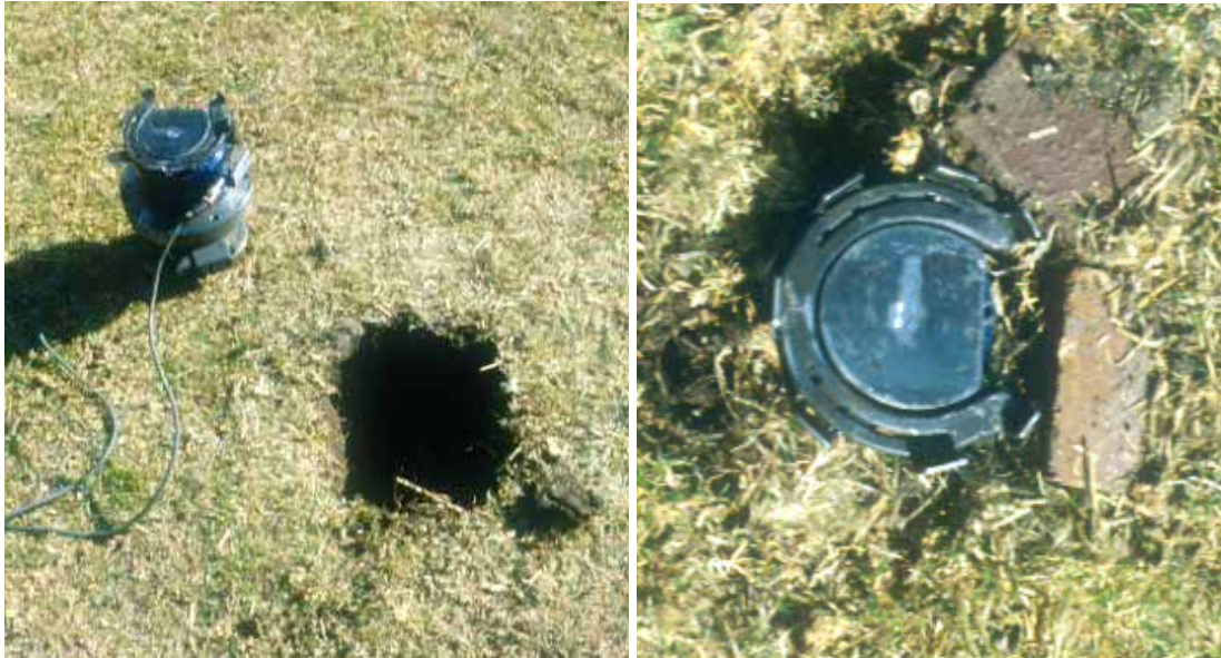
Figure 15: Load cells were buried in a hole, with only the modified shoe and the solar plate visible above the ground. The horse stood on a level surface when one of its limbs was on the test apparatus.
