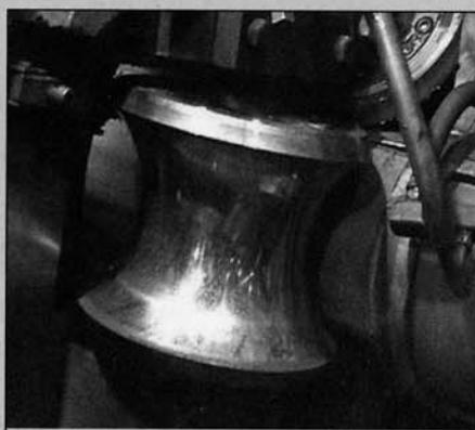
**Figure 3** The edges of the ERW product mentioned in the article are forged together using weld rolls.
