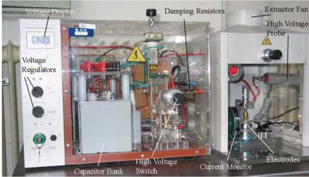
Figure 6.1: Photograph of the electrostatic discharge apparatus used for the various experiments.
