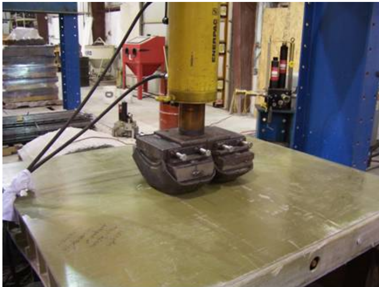
Figure 6.1 Failure Test setup for 5ft by 6 ft specimen
