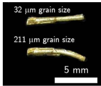
Fig. 1 Samples of pins extruded using the 0.76:0.57 mm die and work pieces having a grain size of 32 \mu\text{m} and 211 \mu\text{m} (modified from [2])
