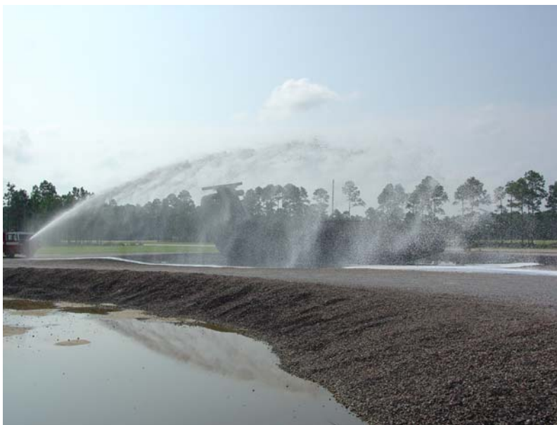
Figure 4.5.3: 300 gpm combined agent Williams Hydro-Chem™ bumper turret nozzle being used for a compressed air foam throw test.
