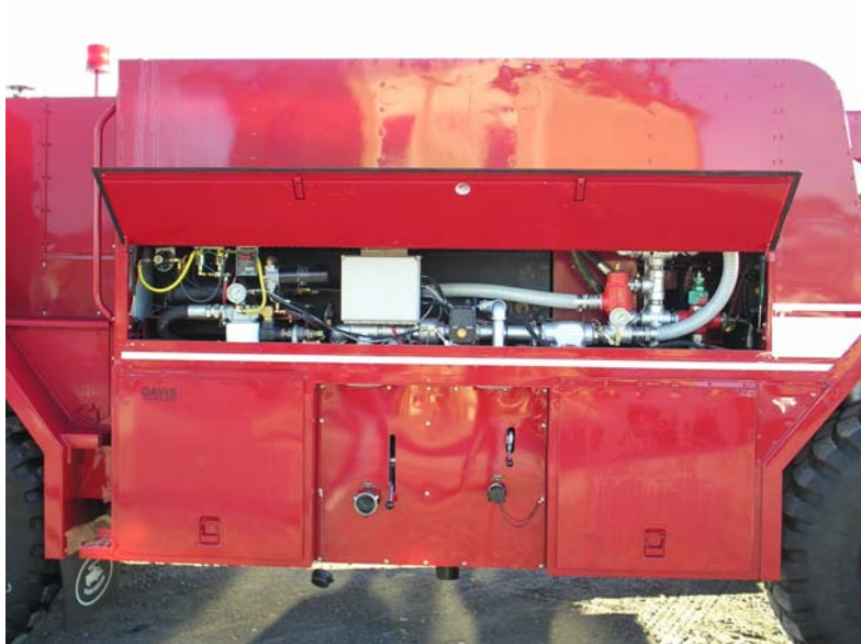
Figure 3.3.10: The UHP P-19's driver's side plumbing.
