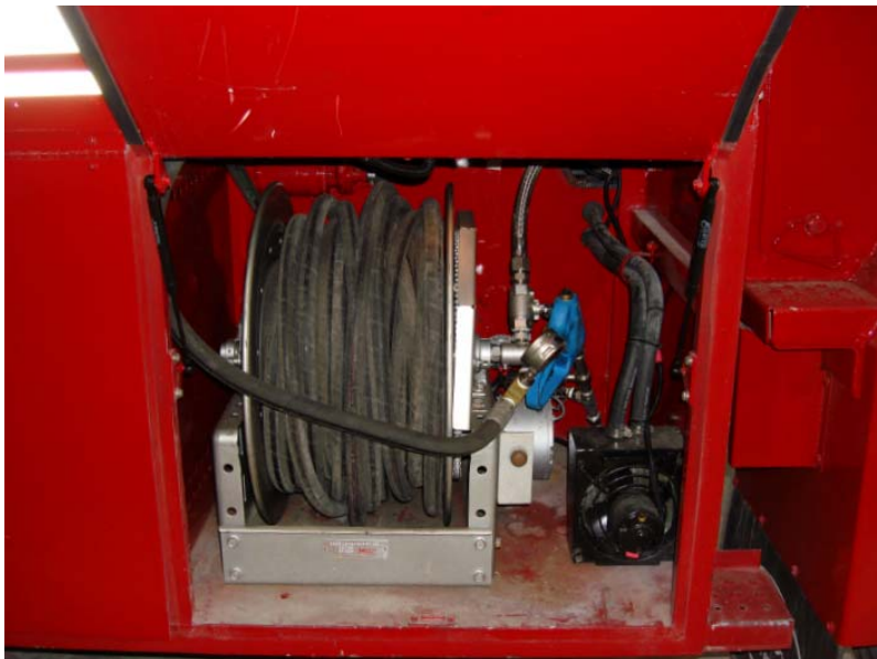
Figure 3.3.11: The UHP P-19's UHP hand line reel.
