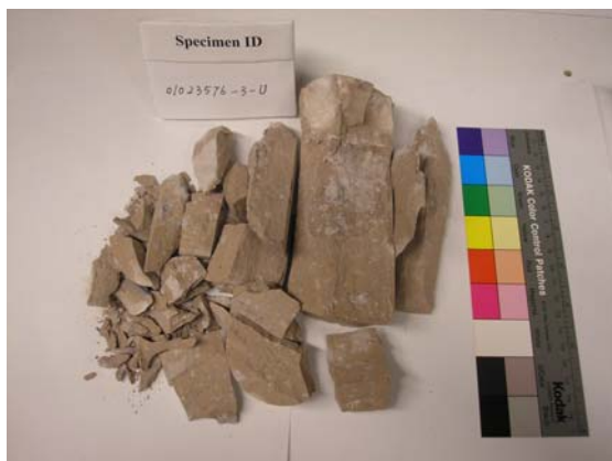
Fig. 5.1: Typical failure at low strain rate (Strain rate= 1.10 \times 10^{-8} )
