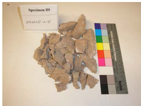
Fig. 5.2: Typical failure at high strain rate (Strain rate= 8.85 \times 10^{-3} )
