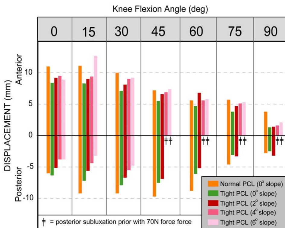
Figure 4-7: Increasing posterior tibial slope was effective at increasing anterior laxity across all flexion angles with a condylar tibial insert. The potential for posterior instability occurred for flexion angles of 45° and higher with 4° and 6° tibial slopes.
