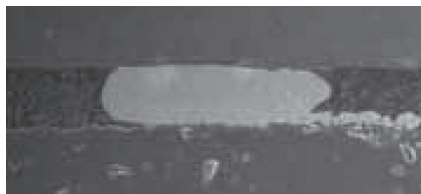
Fig. 5: Cross-section of a gold stud bump, with the top surface flattened by pressure
